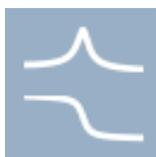
After loading the cantilever and adjusting the detector, find the cantilever resonance by sweeping the frequency of the cantilever drive signal while measuring the detector response signal. The `Frequency Sweep` panel opens when you click the top icon in the work-flow.
